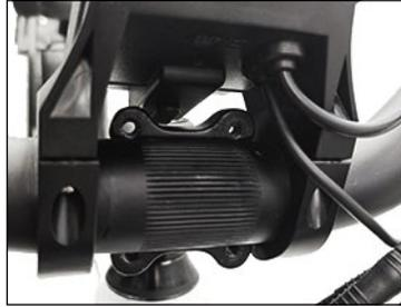
Step 3: Tighten bolts to handlebar stem, but don't tighten completely as you may want to further adjust the angle later to align more precisely. Test the position and adjust the handle bar to your favorite angle. After determining the best position, completely tighten all the bolts on the stem.
