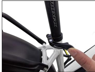
**Warning:** Overextending the seat post can cause it to break or come off your bike, which will put you at very high risk of serious injury or death. Avoid this danger by inserting your seat post into the seat tube far enough that the minimum insertion point is no longer visible. !
