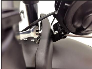
Step 4: Connect the light wire connectors. Pay attention to the arrows on the wire connectors, making sure the arrows align with each other to avoid damaging the interior circuitry.
