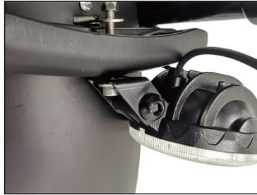
Step 3: Tighten the bolt with 5mm Hexagon wrench and 10mm open-end wrench.
