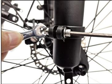
Step 6: Install the rod of front fender in the clamp of the front fork by the screw, nut and washers and then tighten the screw. Install the other rod and make sure the two rods are at the same height.
