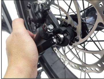
Step 8: Rotate the front wheel. Make sure to fully close the quick release skewer lever on the front wheel and check the wheel balance in Pedal Only Mode. If you notice the riding is imbalanced or the rotation of the front wheel make noise, it means the bolts were not completely tightened or not aligned horizontally.
