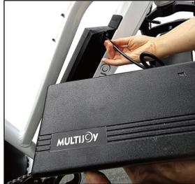
Step 5: Please unplug the charger from your bike and from the power outlet. Please ensure you put the charging port cover back in place to cover the charging port once the battery is charged before you use the bike.
