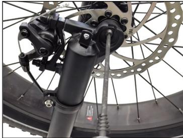
Step 7: Tighten the thumb nut until the quick release lever is held in line with the axle, and then use your palm of your hand to close the quick release skewer.
