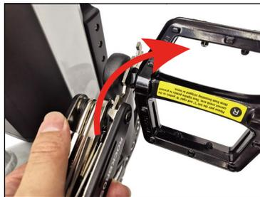
Step 2: Install the left pedal on the left side( the side without chain) and tighten the pedal by 15mm open-end wrench.
