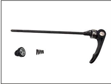
Step 6: Install the quick-release skewer starting from the brake rotor side of the wheel. Inserting the quick-release skewer through and then install the second cone spring on the other side. Ensure the narrow side of both springs towards the wheel hub.
