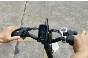
Step3: Turn on the display at the same time, keep holding throttle bar & left brake for 8 seconds.
