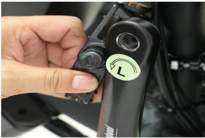
A30. Turn spanner counter-clockwise to fix the pedal L on the left side
