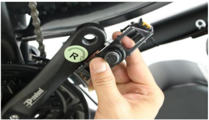
A31. Turn the spanner clockwise to fix the pedal R on the right side
