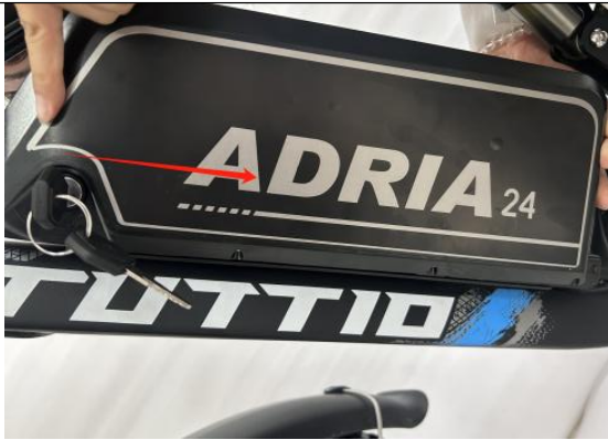
A37. Push the battery downward to install it tightly
