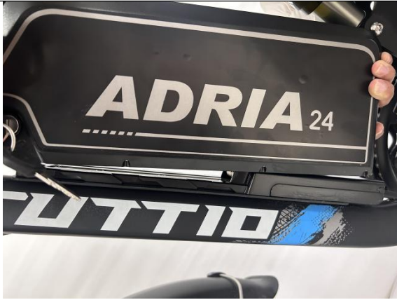
A36. Put the battery on the battery base
