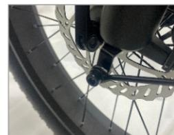
6. Install the fender bracket screws
