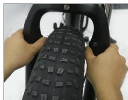
4. Adjust the center position of the tire so that the positions on both sides are the same.
