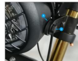
10. Install the No. 5 washer and No. 6 screw as shown in the figure
