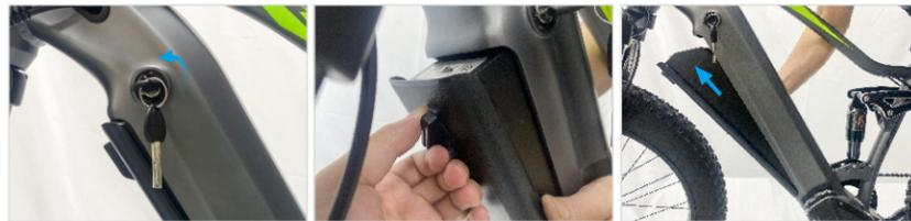
1. Turn the key counterclockwise to open the battery lock
