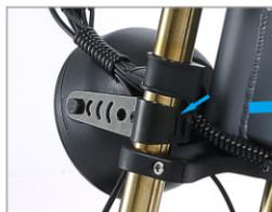
8. Insert the No. 1 fixing piece into the slot of the No. 2 fixing piece
