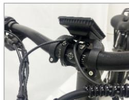
2. Install handlebar riser
