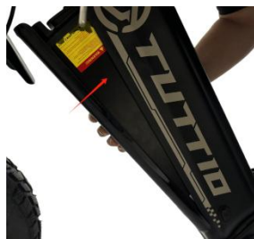
Install the battery
