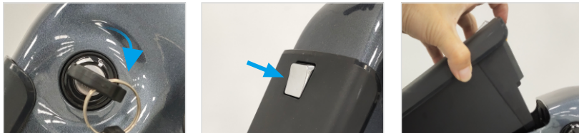
Open the battery lock
