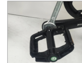
11. Take out the pedal with the letters "R" and "L", align it with the crank hole and lock it with a wrench
