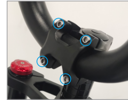
1. Install the U-shaped handlebar
