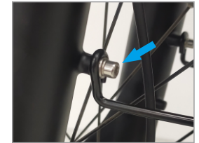
6. Install the fender bracket screws
