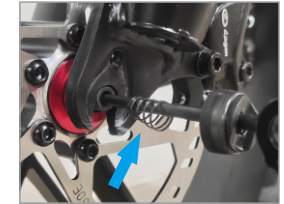
3. As shown in the figure, insert the quick release shaft into the tire shaft and install the other nut and spring properly
