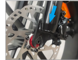
2. Install the front fork on the front wheel bearing
