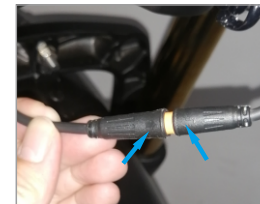
10. Connect the light cable (note that the direction of the arrow needs to correspond)
